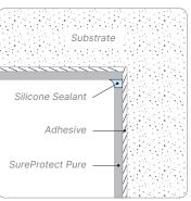
Thermoformed External/Internal Corner
